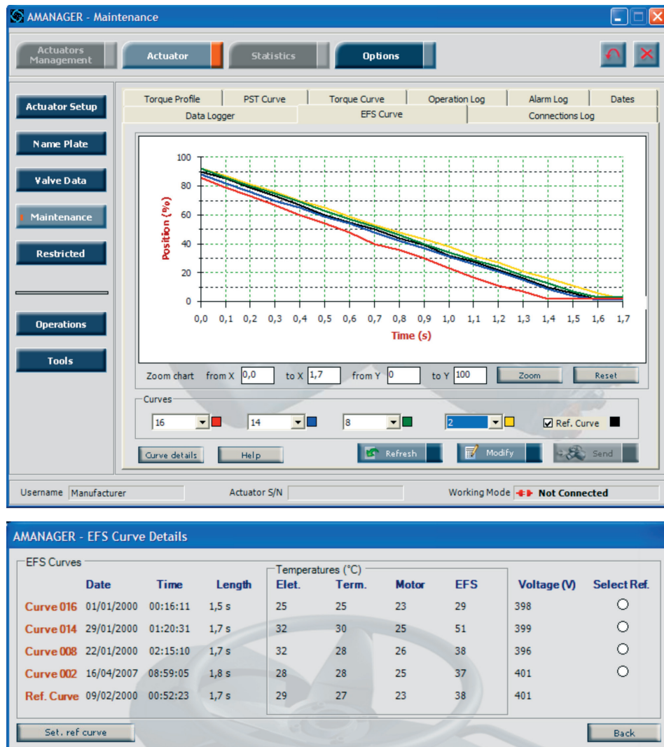
Figure 50. Emergency Shutdown Graph
