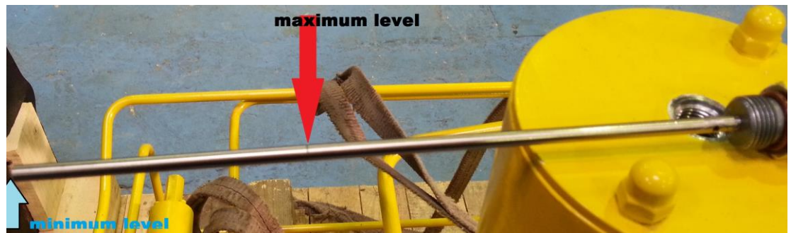
Picture 18 – Level measuring stick
