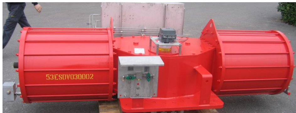
Picture 8 – Actuator with two cylinders
