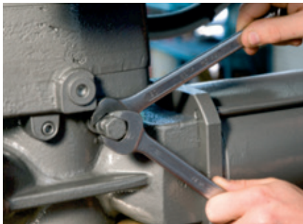
Adjusting the stop screw positioned on the actuator housing
