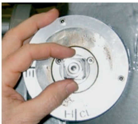
5. Rotate the indicator nut clockwise until it blocks at the end of the threads; rotate a few degrees counter clockwise until the flat surface is perfectly aligned with the CLOSE indication of the label.
