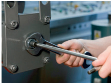
Adjusting the stop screw positioned on the spring cartridge end flange
