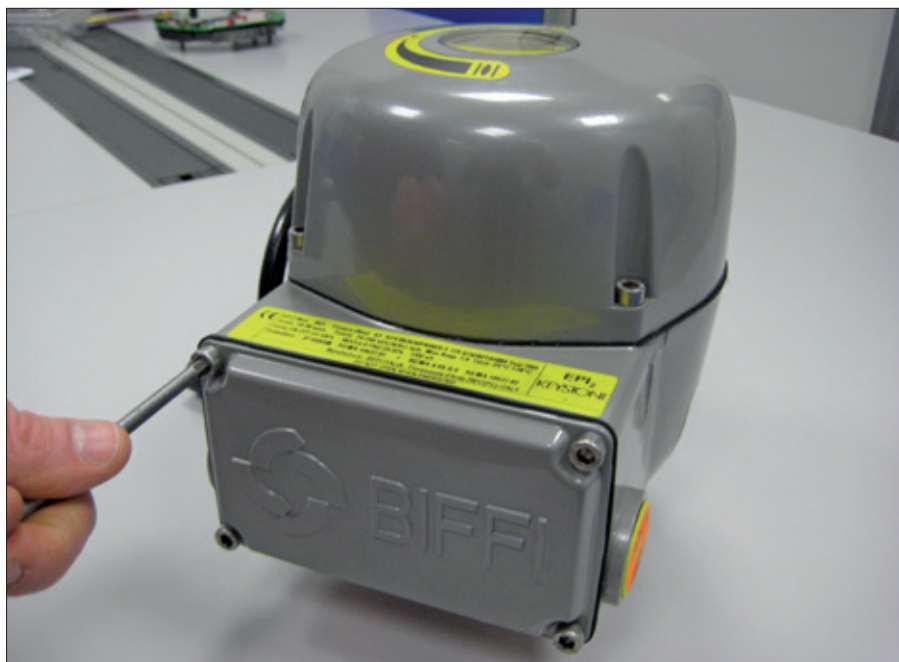
FIGURE 10 - Removal of the terminal board enclosure.
