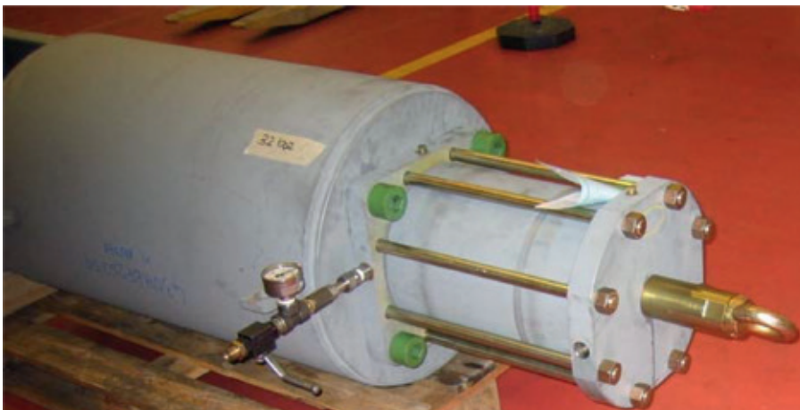
FIGURE 9 Mechanical stop on cylinder end flange
