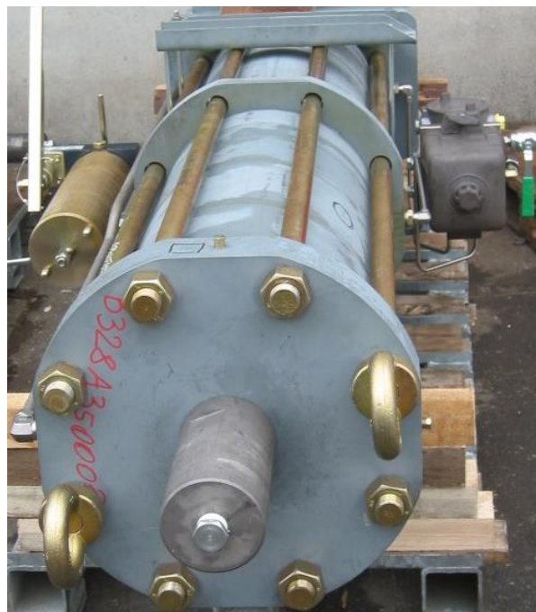
Picture 6 – Mechanical stop
