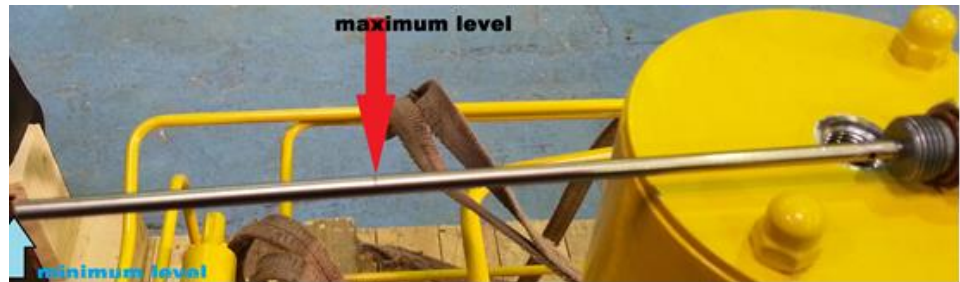
Picture 13 – Level measuring stick
